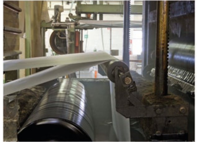
The two reinforcing inserts are impregnated, then coated.
