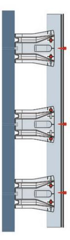
Subject to specifications, support profiles are installed storey by storey in lengths of 3 meters. A fixed point should be placed in the center of the profile, followed by 2-3 sliding points on either side. Special care must be taken to ensure that the joints of profiles and cladding panels are aligned. Cladding material must under no circumstances be mounted across a joint between profiles.
