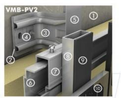
HANGER SYSTEM 2-layer substructure
