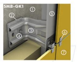
**CLAMP FIXING** 1-layer substructure
