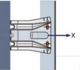
Combining different lengths of SPIDI<sup>®</sup> wall brackets is an easy way to compensate for even large wall-to-panel distances as well as protrusions or recesses in sections of the facade, as are often found in renovation projects. These kinds of applications truly benefit from the SPIDI<sup>®</sup> wall bracket's excellent lateral and torsional stability.
