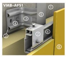
HANGER SYSTEM 2-layer substructure
